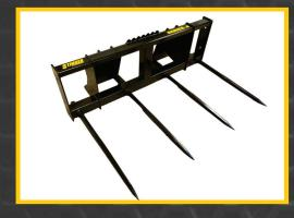
The Stinger Attachments Series 4 Bale Spear is designed for large machines. It has the ability to move 2 large bales at a time to increase efficiency. The 61" spacing is designed for large square bales and the 100" spacing is designed for large round bales. This mover features 4 spears spaced evenly with an outer spacing of 61" or 100". This design penetrates and moves large square bales fast and efficiently.
