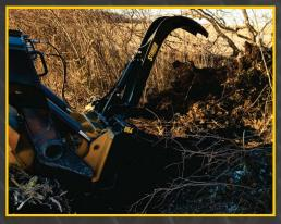
The Stinger Attachments Stump Grapple has all the same features of the Stump Bucket with the added versatility of the grapple. The added grapples aids in clamping onto debris such as roots, rock and stumps and assists with removal in both digging and relocating stumps, roots or rocks. This grapple is built to handle the toughest jobs.
