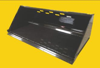
The Stinger Attachments Snow Bucket offers a high capacity with high strength. This bucket is designed to move large amounts of snow fast and efficiently. It has a top 4" x 2" tube and a rolled insert bottom-radius support for added reinforcement and easy cleanout. The sides are ¼" thick and have ½" x 3" steel supports. These buckets also have a see-through design to allow the operator better visibility. to get the job done with speed and ease.
