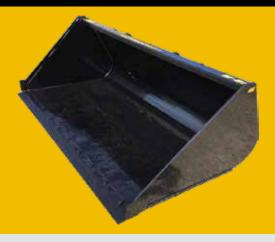
The Stinger Attachments Liquid Slurry Bucket is ideal for liquid slurry type products. This is an extremely high volume bucket that is designed to carry a full load of liquid slurry. The 60 degree back angle allows for increased rollback, which enables the operator to level the bucket edge for maximized liquid carrying capacity.
