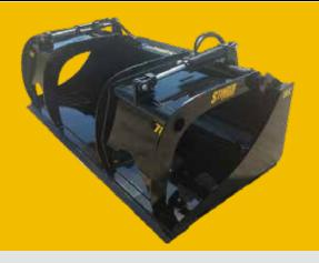
The Stinger Attachments DG Series Demolition Grapples are designed for both large and small debris. The solid bottom and wide grapple opening ensures the most capacity carried with every load. The curved side plates allow the operator to clamp onto large objects like logs and scrap. Our demolition grapple bucket also has an added rolled insert bottom-radius support. This feature strengthens the shell and aids in easier clean out.
